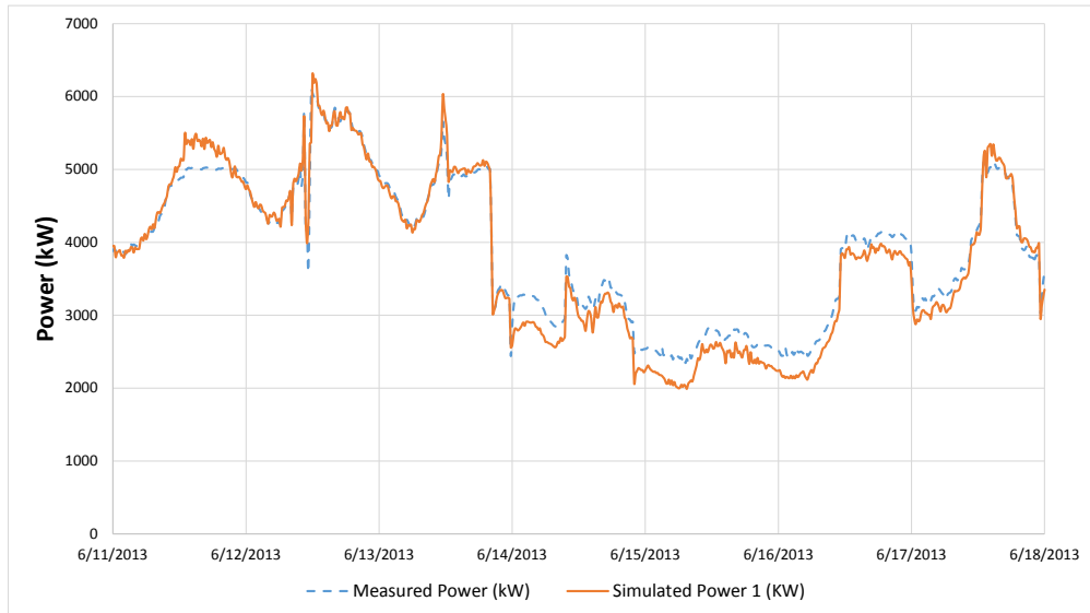
Figure 66 Plant Power Consumption Simulation vs. Measured
