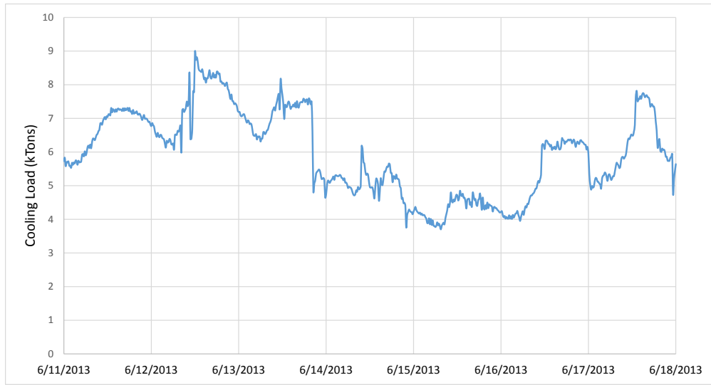
Figure 65 Cooling Load Profile during Validation Week
